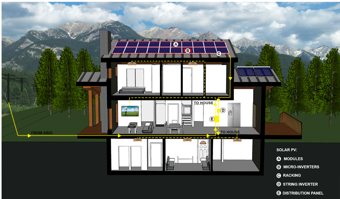
Figure 3: Solar PV Equipment
